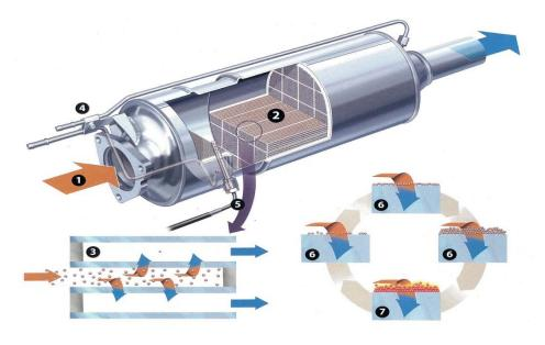
Exhaust gases enter the DPF 1 and pass through the silicon carbide core 2. The core is designed to have an enormous surface area relative to its compact external dimensions and collects any soot particles present 3
